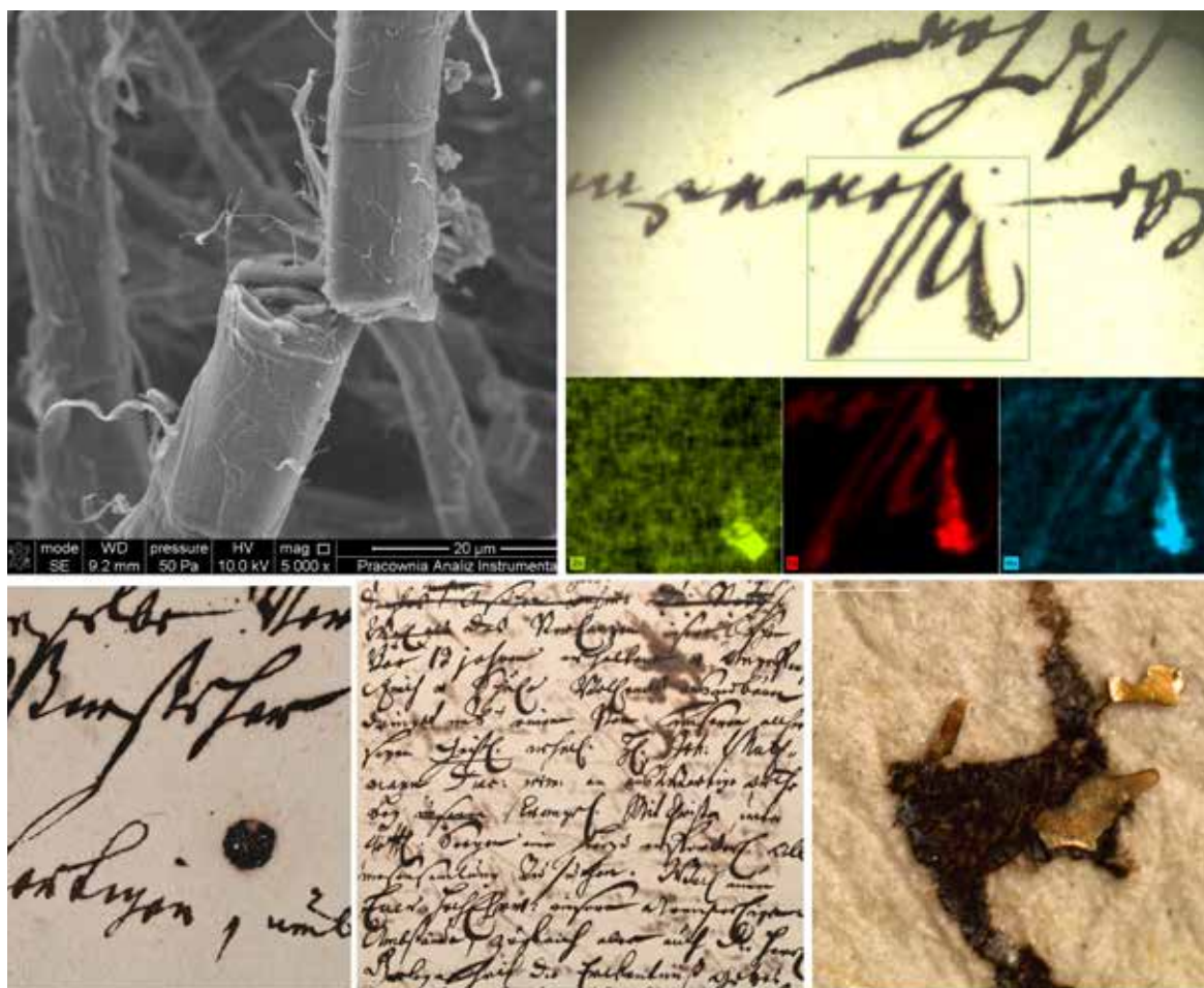
Mica flakes and brass particles derived from blotting sands identified in iron gall ink through analytical examination, from the collection of the Evangelical-Augsburg Parish in Kraków.
