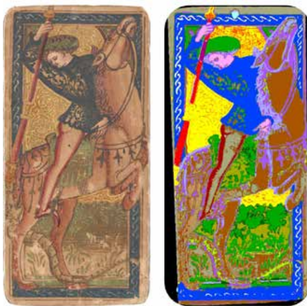
Visible-light photograph of the Knight of Wands tarot card (©C2RMF, L. Clivet), alongside a clustering-based representation of the same card derived from analysis of a multimodal data cube combining three spectroscopic techniques (RIS-VNIR, RIS-SWIR, and XRF-2D) (©C2RMF, L. Pagnoux, E. Laval, K. Laclavetine, R. Moreau; ©LAMS, L. de Viguierie, L. Brunel).
