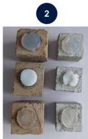
Assessment of the desalination efficacy of natural hydrogels in the laboratory
